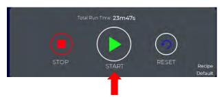
The center button will change from START to WARMING, and the button boundary will change from solid white to flashing green to indicate the system is warming up.
