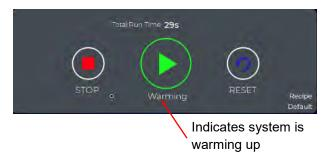
When the center button changes from WARMING to READY the pumps will automatically pressurize the system to the desired setpoint.
