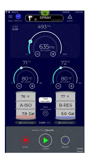
3. Check the A-ISO and B-RES fluid levels using a dipstick and enter the amount by pressing the respective drum icon on the screen.
