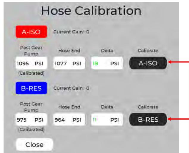
Press to calibrate A and/or B pressure sensors
