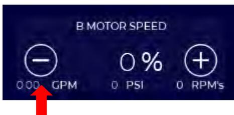
11. Press the START button to begin purging and heating. Note, there is no warmup cycle in Exchange Mode. If the material needs to be heated before turning pumps on, set motor speed to 0% or run at low speeds until fluid is warmed. Otherwise fluid will be heated during pumping.
