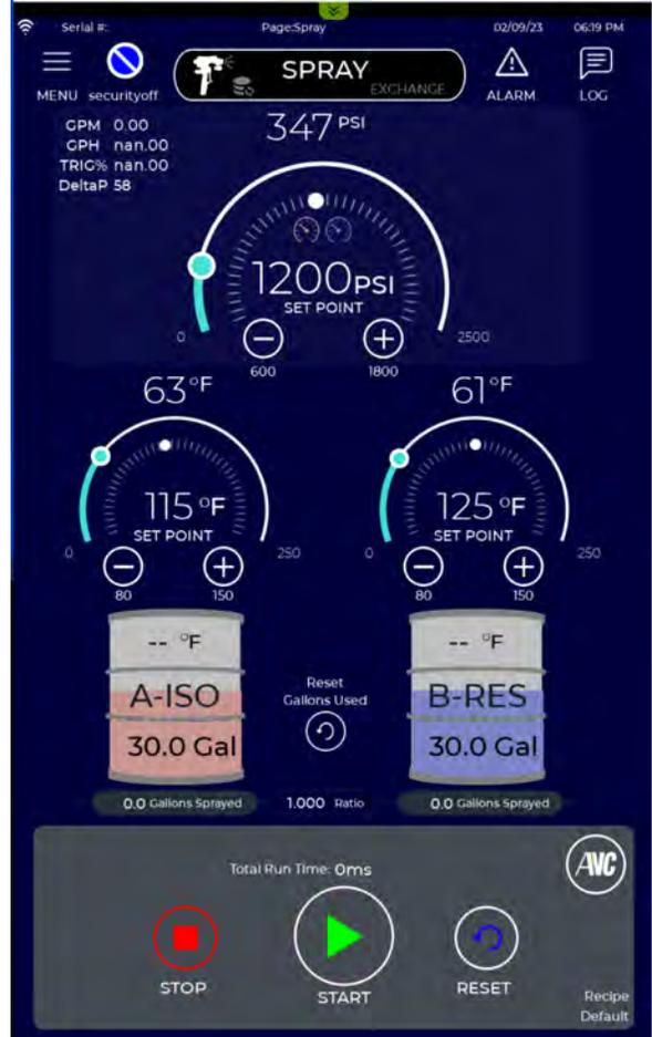
3. Check the A-ISO and B-RES fluid levels using a dipstick and enter the amount by pressing the respective drum icon on the screen.
