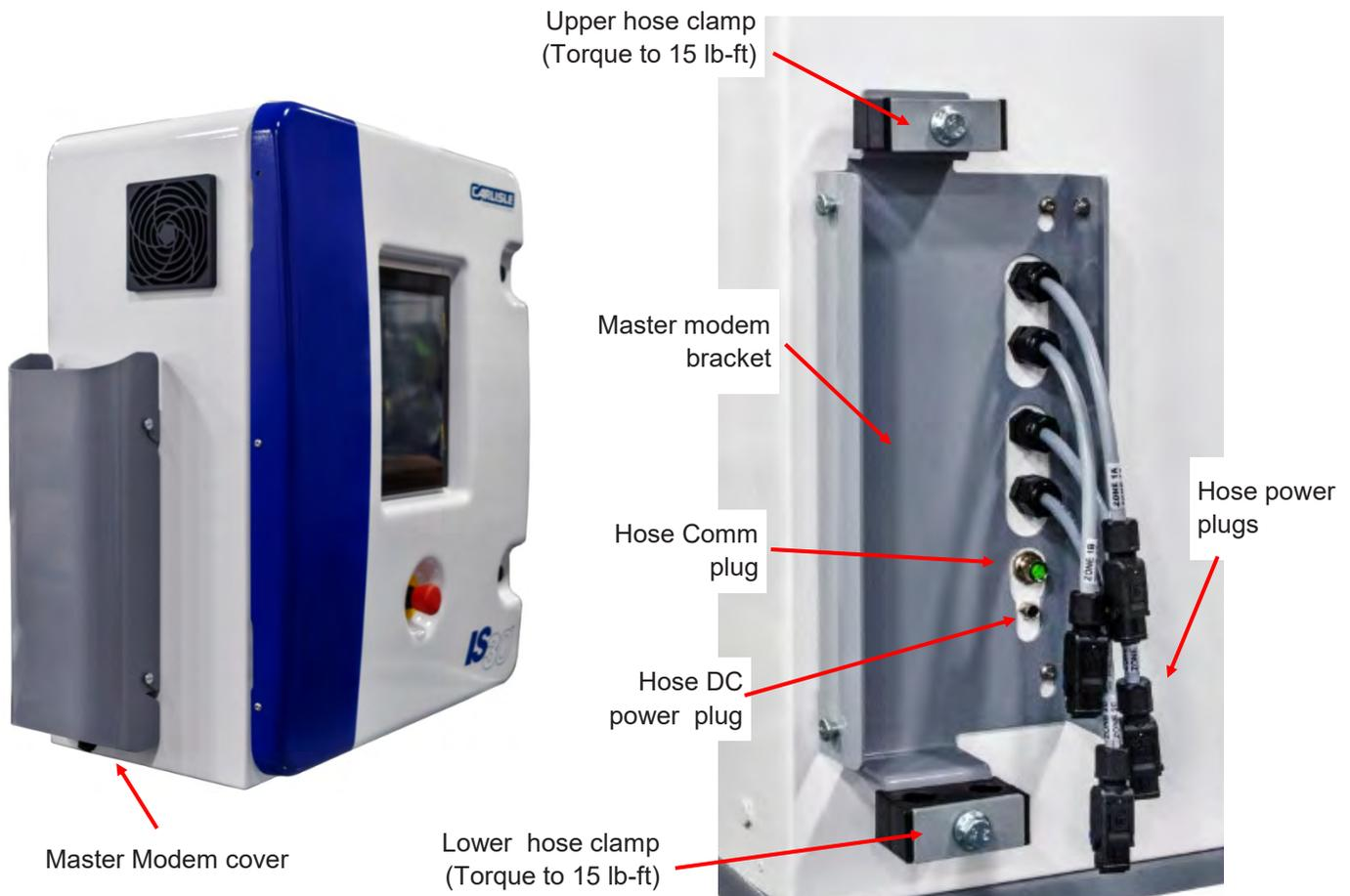
Lift and slide the Master Modem cover off its bracket. Remove upper and lower hose clamp bolts and outer clam shells. Set the Master modem in place in its bracket. Note: using zip-ties can help to hold the modem in place when attaching hoses.
