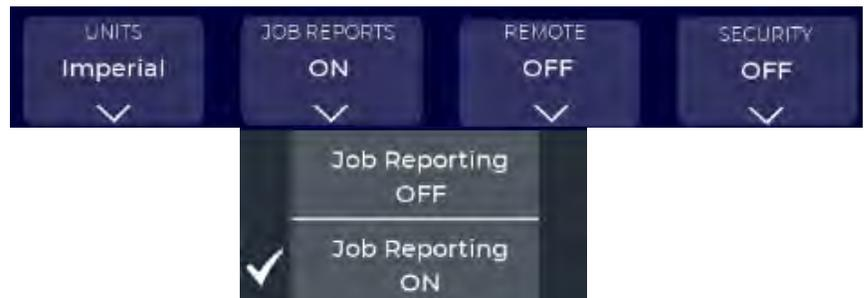
**REMOTE SERVICE:** This allows remote access by authorized persons for monitoring and/or control of the IS40. This must be ON to perform remote service and/or remove control. See page Section 28 for more information on Remote Service.
