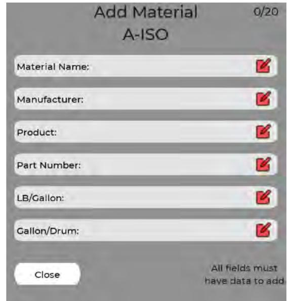
To edit an existing material select **Edit Material**, select the material to edit from the drop-down menu, and enter new values as required.
