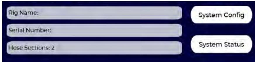
Pressing the **System Config** button opens a window that allows a user with administrative privileges to change Rig Name, Serial Number, and Unheated Whip Length. Other pertinent system information (firmware versions, hose lengths, serial numbers) is shown, but cannot be changed. Use the arrow buttons to move between pages. Firmware can be updated from a USB memory stick using the Firmware Update feature on the second page.
