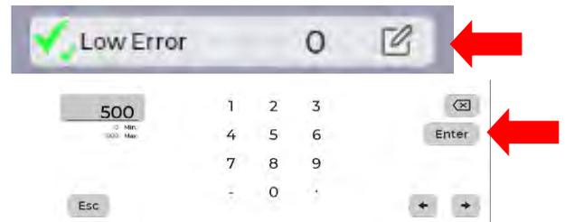
After entering these changes, the Pressure Parameter Table for the selected Recipe will show the new value of 500 psi. To activate this change, the press the LOAD button.
