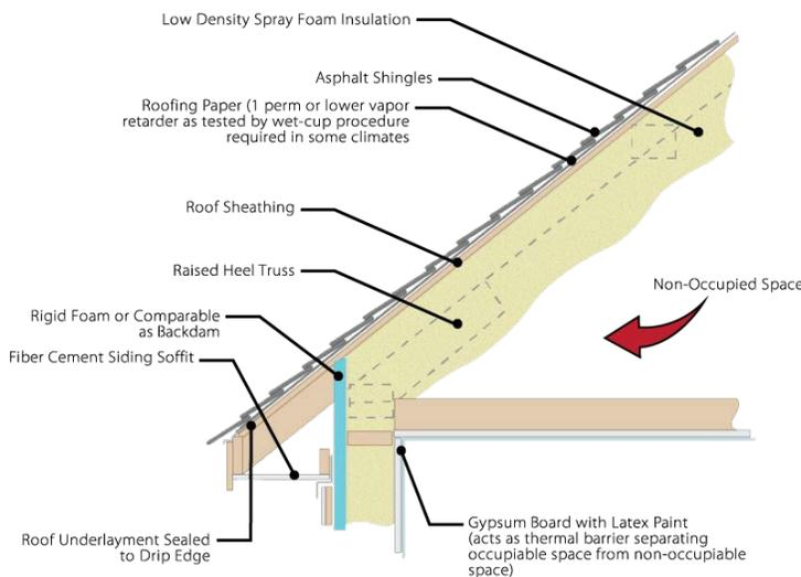
In unvented attic assemblies, the thermal envelope is continued from the lower-level walls up through the energy plates and risers (knee walls) onto the underside of the roof sheathing to fully encapsulate the attic space. The floor of the attic is left uninsulated. All soffit, ridge and gable vents are eliminated. The attic is now considered a component of the conditioned space. The drawing below illustrates an unvented attic assembly.
