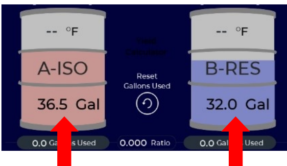
Press on A or B drum icon to open material input window
