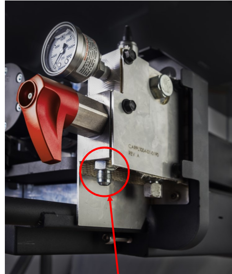
Recirculation hose fitting (JIC 5 A, JIC 6 B). Use kit PN 341133 to connect to 1/4" NPT fittings if required.
