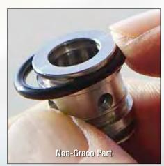
After spending the same amount of time submersed in solvent, the Graco O-ring (left) still fits snugly, protecting the side seal, while the non-Graco O-ring (right) expanded in diameter and swelled in cross section.
